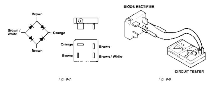
Circuit inside of the diode rectifiers is as shown in Fig. 9-7. Check continuity between each terminal by using a circuit tester as shown in Fig. 9-8. The rectifier is normal when condtinuity is as follows:
